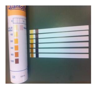
If the warning field just above turns blue/purple during the reaction time of 45 seconds, the hydrogen peroxide concentration is greater than 2000mg/L (outside the measuring range of the test)
